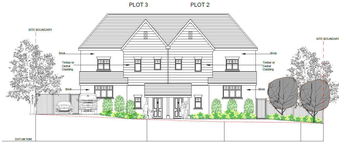
Front Elevation (West)
